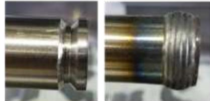
Initial plug insert and as-deposited material for end cap
