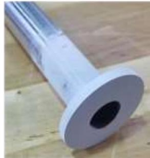
Flange with die penetrant showing no surface-connected voids
