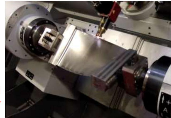
Repair of a gas turbine blade edge\*
