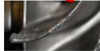
Pre-machined re-tipped turbocharger impeller\*
